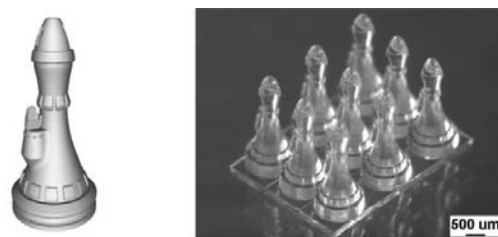
(b) Micro-bishop CAD model and fabricated array
